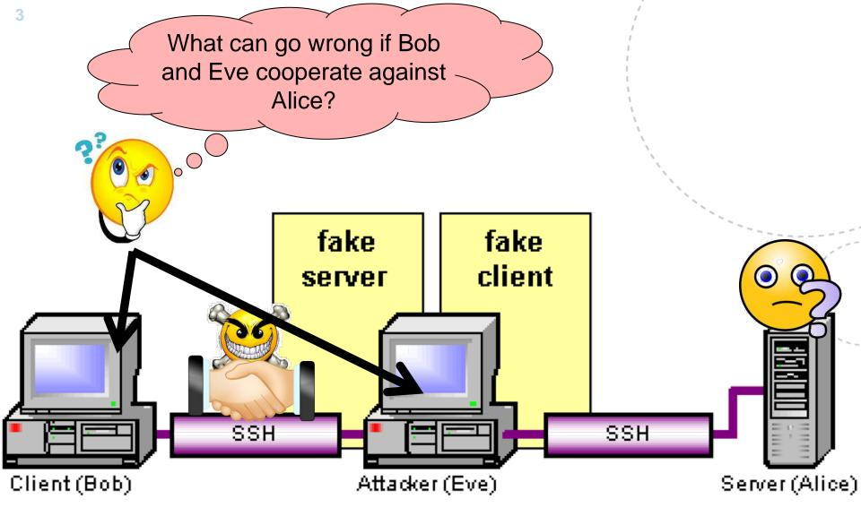
A typical setup of a Man-In-The-Middle attack (rouge proxy server with SSL)
