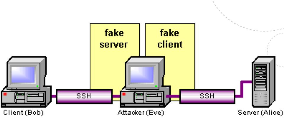
A typical setup of a Man-In-The-Middle attack (rouge proxy server with SSL)
